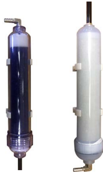
Air Drier Cartridges. Changes from blue to red color when it needs changing.
